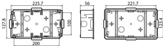
**Сборка и монтаж / Assembly and installation (mm/mm)**
