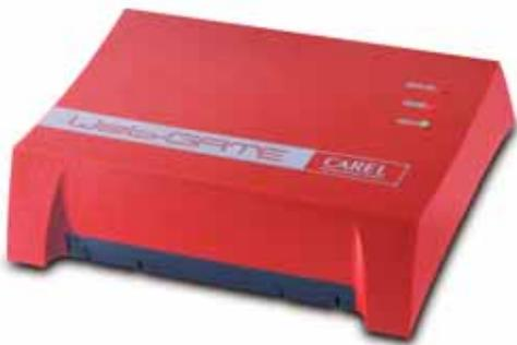
Using Web-GATE, the individual controllers can also be economically connected to Ethernet™ networks and consequently exploit the power of the TCP/IP protocol.
