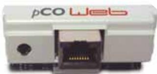
pCO Web is a board for the pCO sistema controllers that interfaces the latter with the emerging protocols (BACnet™ and SNMP) in HVAC, and is based on both the physical Ethernet™ and EIA-485 standards.
