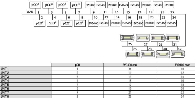
Below is a diagram with the EVD400 driver in a tLAN connection, while the others components are connected in the pLAN:
